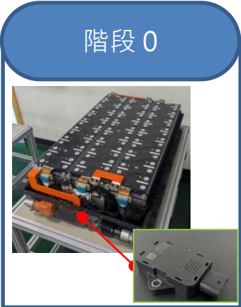
Temperature & Hydrogen Gas Sensors
